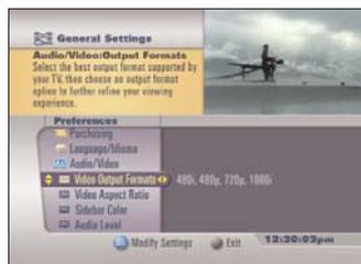
To display the General Settings menu, press the **SETTINGS** key, then press **▲**. (If your service includes the QuickMenu™, you could alternatively press the **MENU** key twice.)
